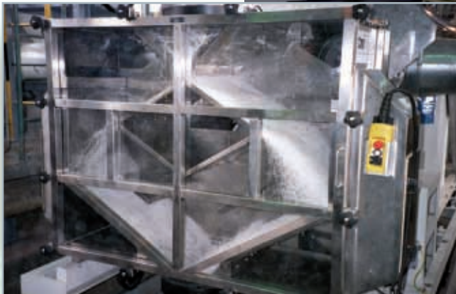
P800 DeDuster cleaning 40 T/H with LDPE while loading railcars
