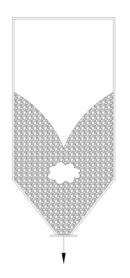
The compressed air forces the lime below it and, if there is no positive feed control below the silo, the mixture of fine and coarse lime will be forced through the feeder into the slaker. This sudden introduction of a large volume of lime into the slaker will produce a violent reaction releasing steam that would act as an explosion spraying hot slurry out of the slaker. There is no way to guarantee this accumulation of powder will never occur in any silo.
