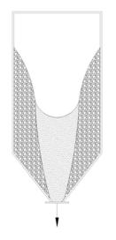
When lime is fed from the silo, first the fine particles from the center will exit the silo. As the height of the fine material in the center is reduced, some coarser material at the perimeter of the silo will collapse into the center of the funnel and trap a large air pocket in the cone of the silo.
