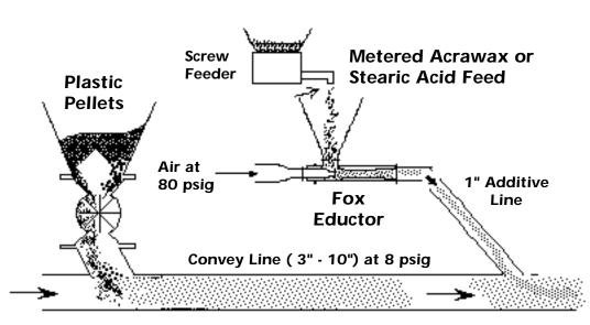
Additive Injectionwith no moving parts
