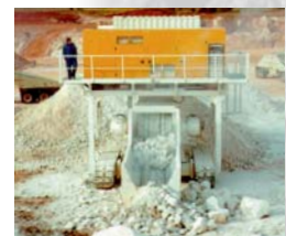
Autarker raupenmobiler Gipsbrecher direkt an der Abbaufont Self-powered track-mounted gypsum crusher directly at the face
