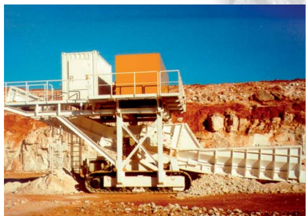
Autarker raupenmobiler Gipsbrecher direkt an der Abbaufont Self-powered track-mounted gypsum crusher directly at the face
