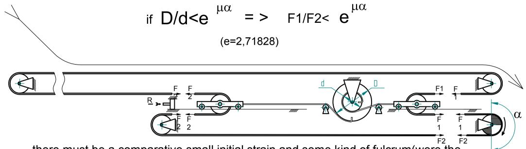
there must be a comparative small initial strain and some kind of fulcrum(were the reaction force R is shown). This fulcrum have to prevent the full loosen of the belt when the conveyor is stoped.
