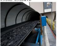
**First to pass the test** – Goodyear Engineered Products SHIELD<sup>TM</sup> underground conveyor belt compound is the first to receive the MSHA certification for flame resistance while also reducing smoke-density and toxicity.
