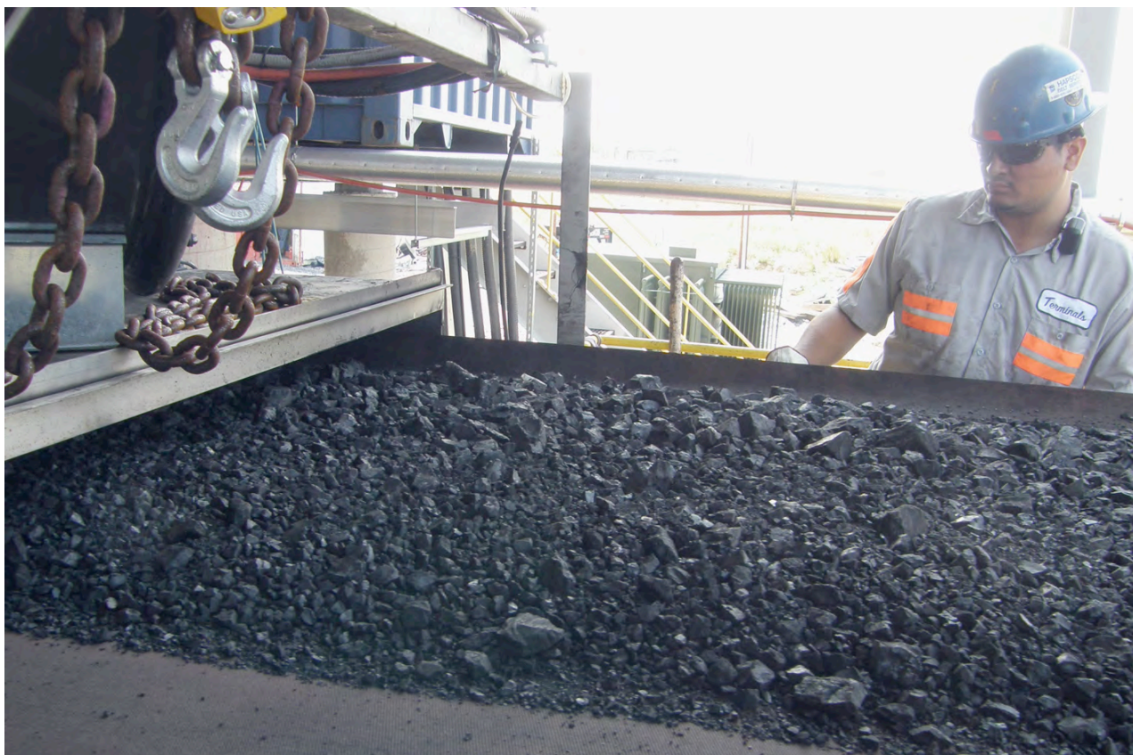
Figure 9 MW-dried coal emerging continuously from the drying zone
