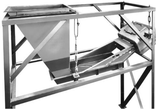
The tray on this feeder is slotted at an angle to spread material evenly over a conveyor belt which will be installed at right angles to the tray.
