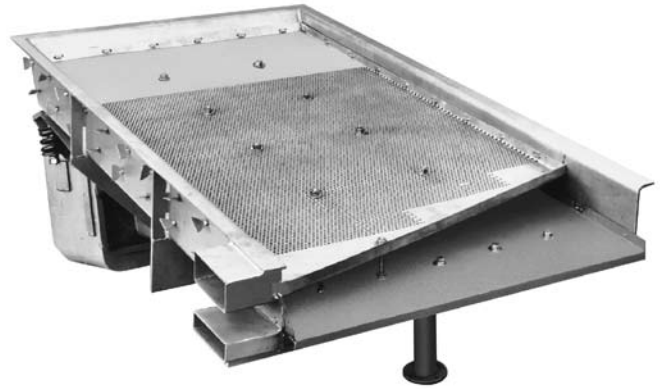
A three-deck screening feeder discharges oversize and undersize products to one side while the desired material flows off the end.
