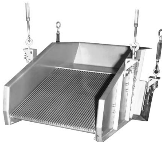
Feed with a rod-deck screen. These are well suited for materials where water is present.
