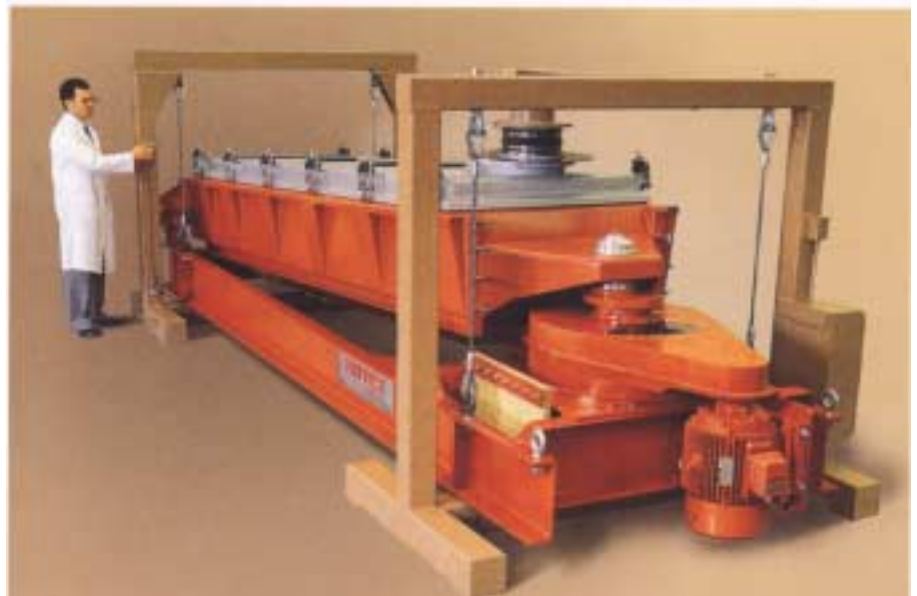
Model 54 DA ROTEX Screener equipped with Dynamic Absorber Drive. Machine is cable suspended on cable-support stand, and also features the ROTEX Slider Inlet. (Drive guards removed for clarity. Do not operate any equipment without guards installed.)
