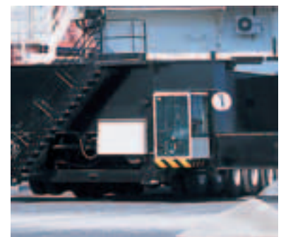
Additional cab on the chassis
