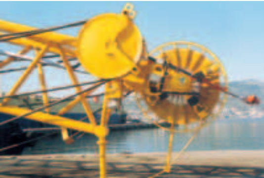
Cable reel on the boom head
