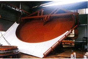
Frigate delivered a pelletization disk of 30 TPH of 4.5 m dia with a rotating speed of 9 rpm
