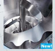
SinConvex® spiral blade (patented) driven and supported from above with the advantage of complete discharge.
