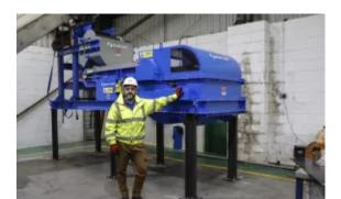
Drum Magnet and Eddy Current Separator Module at HML Recycling (Photo: ©Bunting Magnetics Co.)
