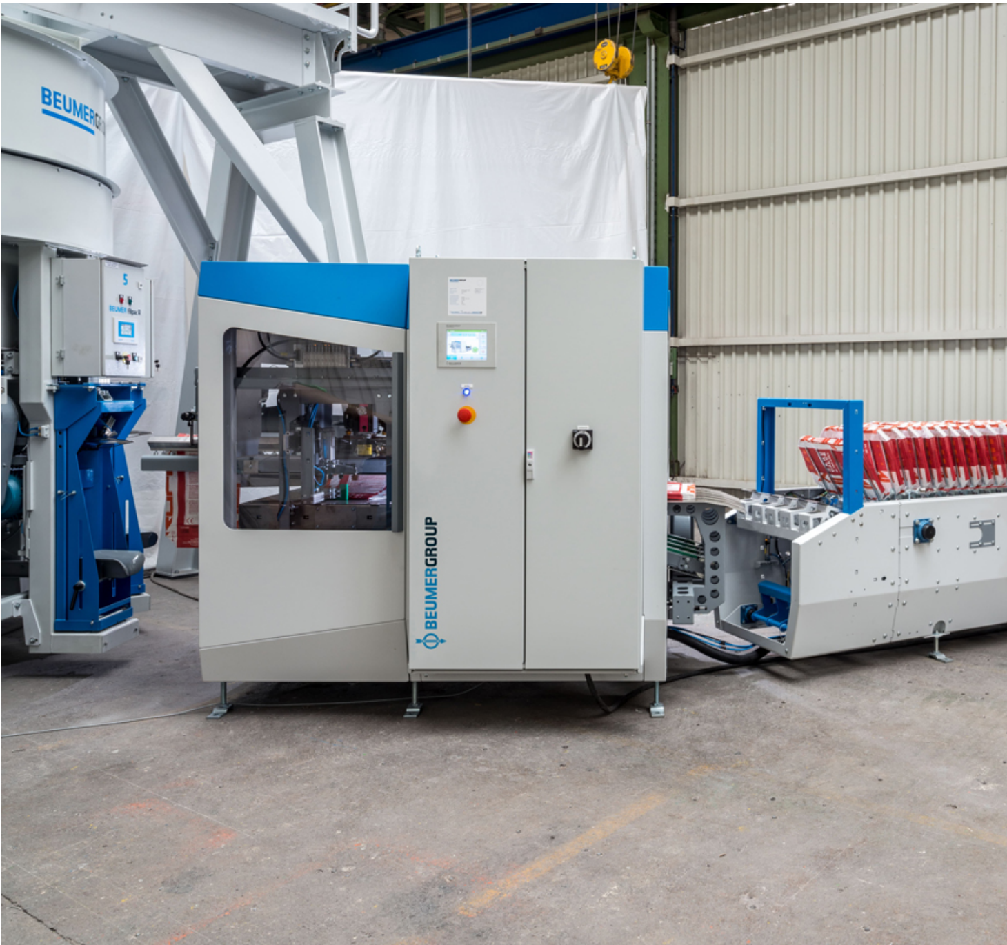
Fig. 2: The gripping system and the application unit apply the bag from the bag ream safely onto the filling spout.
