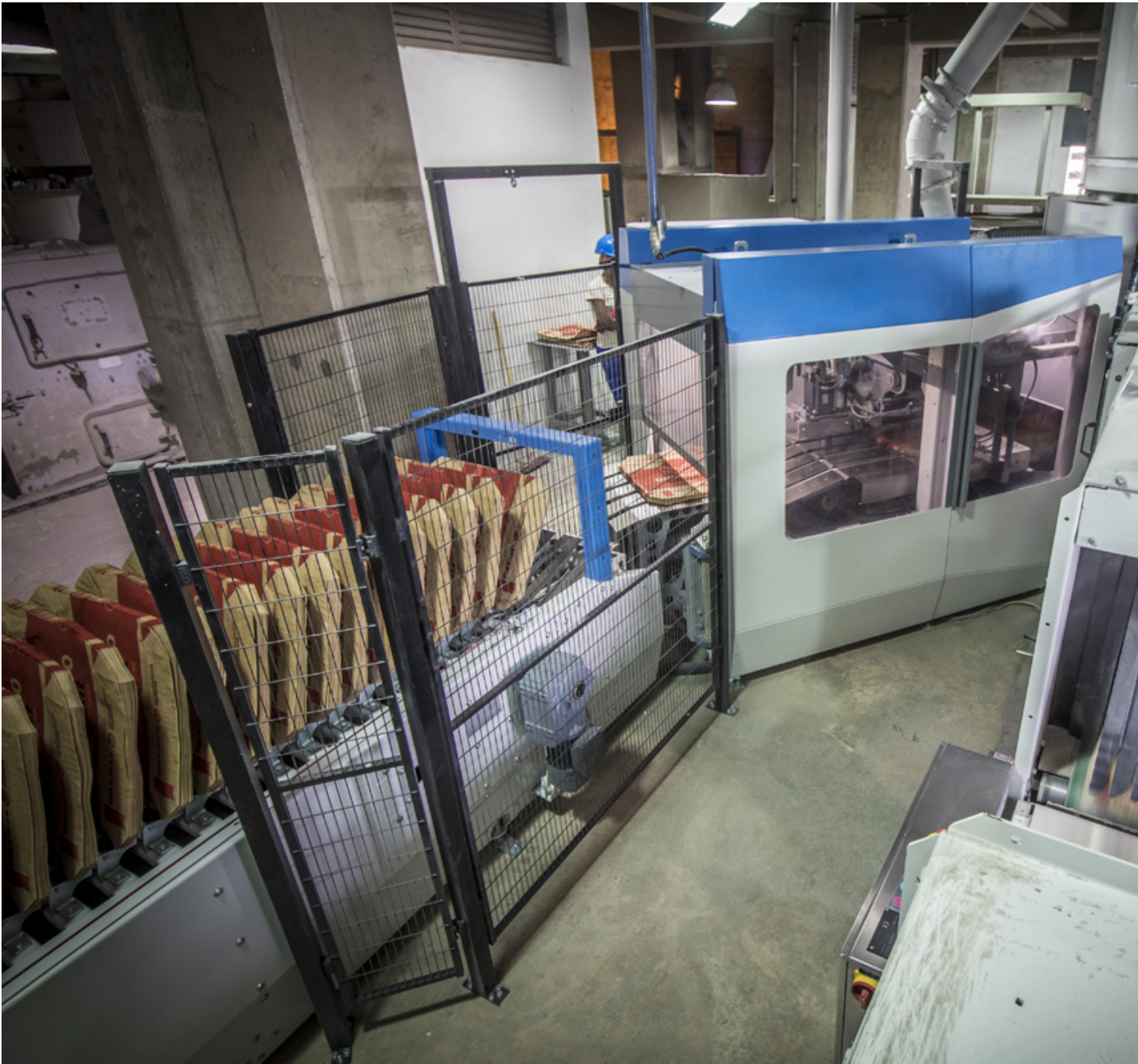
Fig. 1: Capacity and efficiency of the BEUMER fillpac can be further increased with the BEUMER bag placer and the ream magazine.
