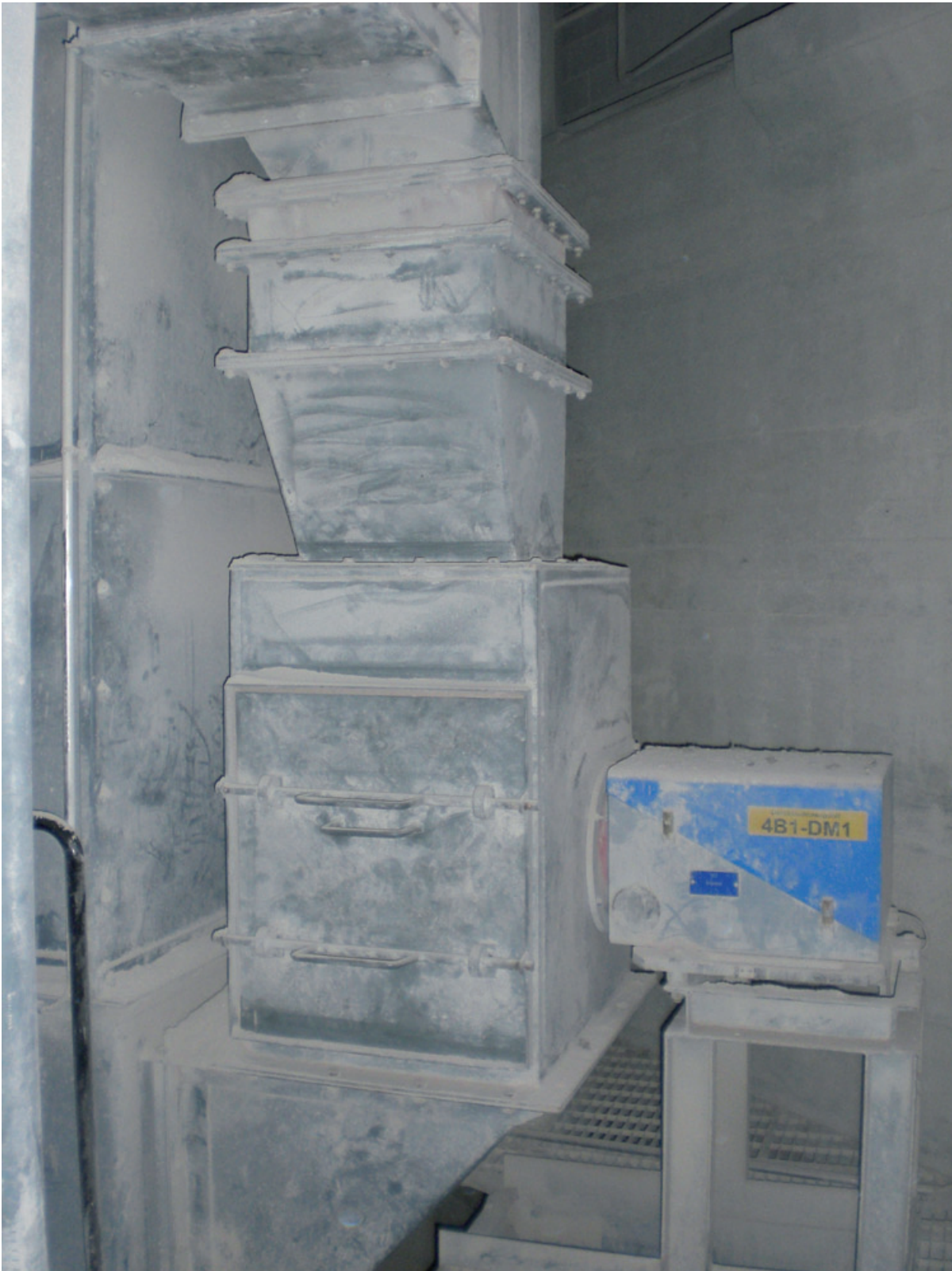
Previous mass flow measurement system with baffle plate
