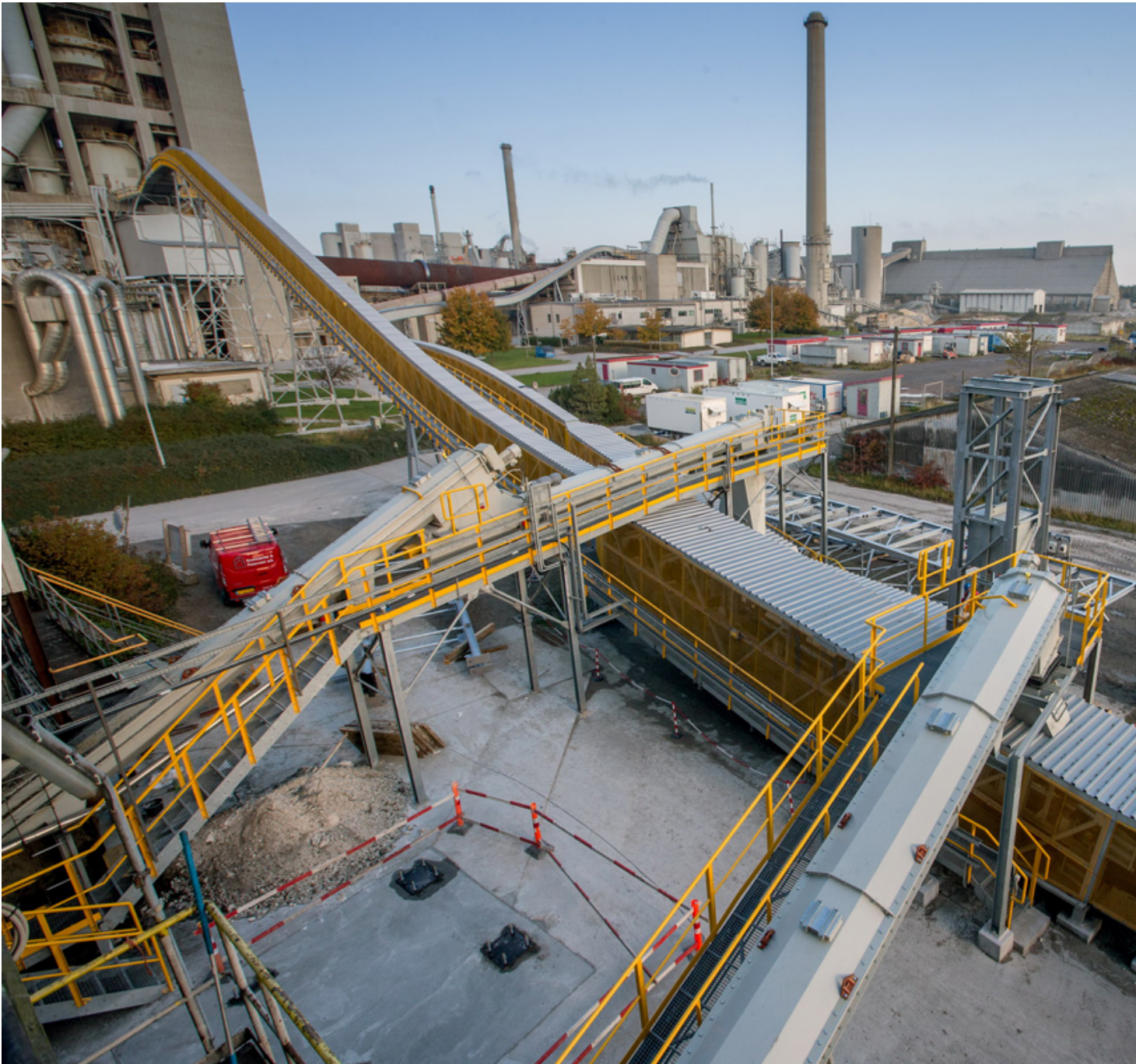
Fig. 1: BEUMER Group supplied a single-source system to Aalborg Portland to feed the calciner and the main burner with alternative fuels and raw materials. The main component is given by the Pipe Conveyors. They are fed via screw conveyors.
