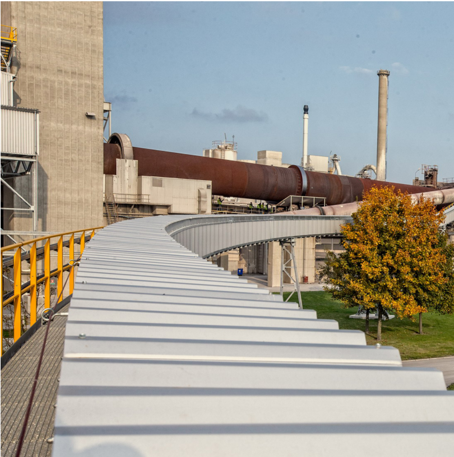
Fig. 4: The Pipe Conveyor conveys the material directly to the rotary kiln. Curves can be easily realised during construction.
