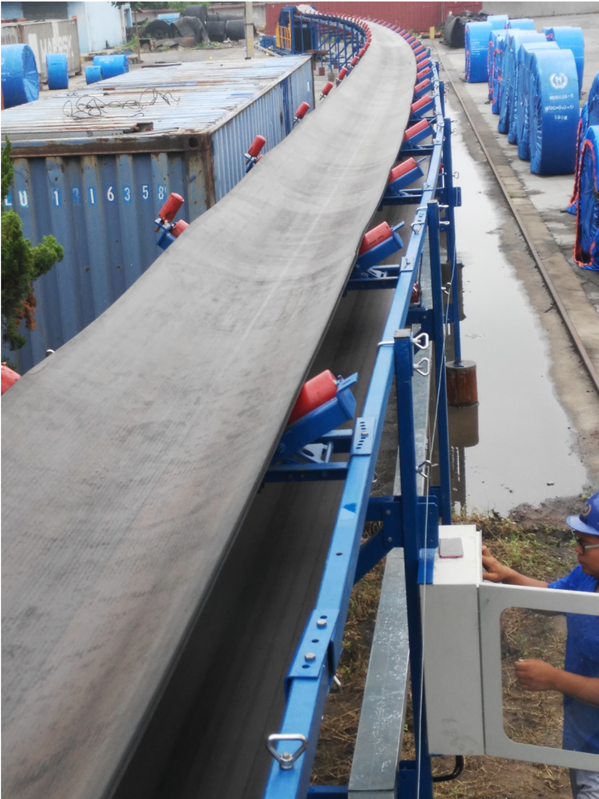
Huaxia_HHE conveyor belt. Min. radius 300m
