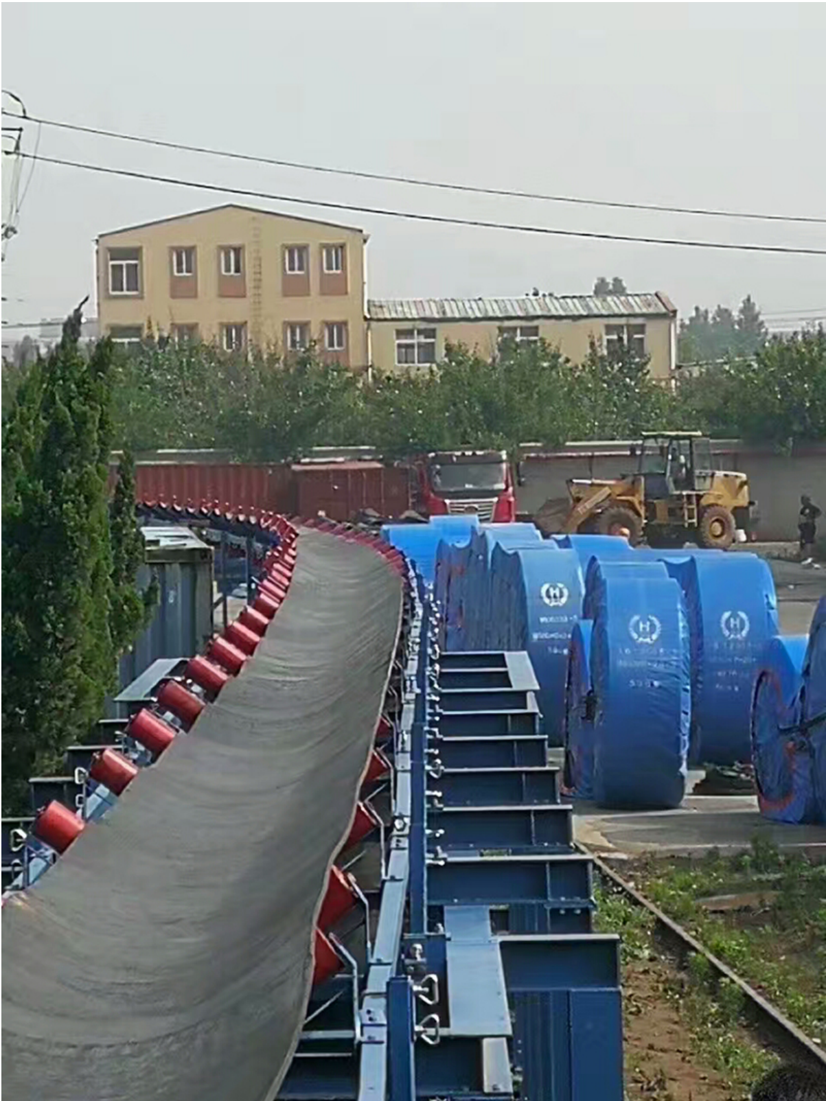
Huaxia_HHE conveyor belt. Min. radius 300m
