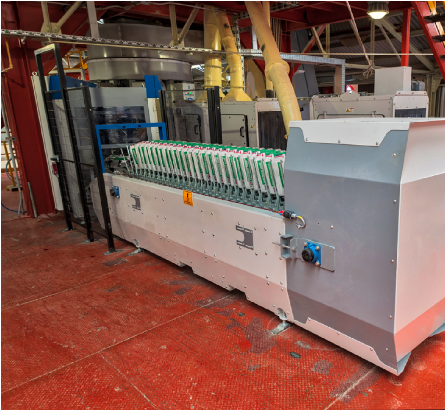
Picture 4: The BEUMER fillpac R is equipped with a ream magazine for 700 bags
