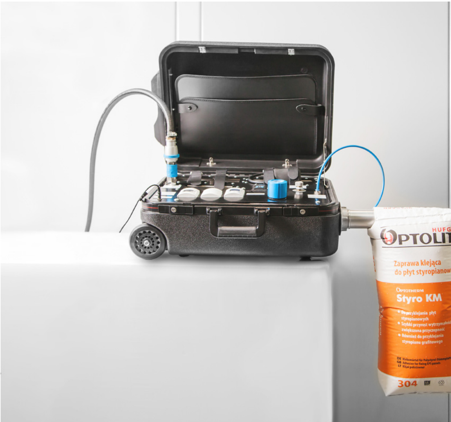
Picture 1: The BEUMER bag tester enables users to exactly determine the venting capacity of any type of valve bag.
