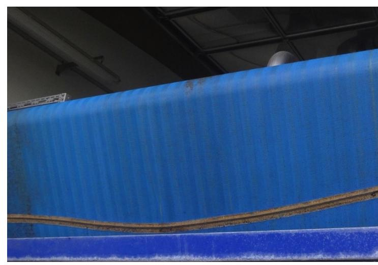
Besides efficient dewatering, the key factor of the GKD-belt Type 1003 with integrated wear indicator is a reliable PAD seam. (Picture: ©GKD)
