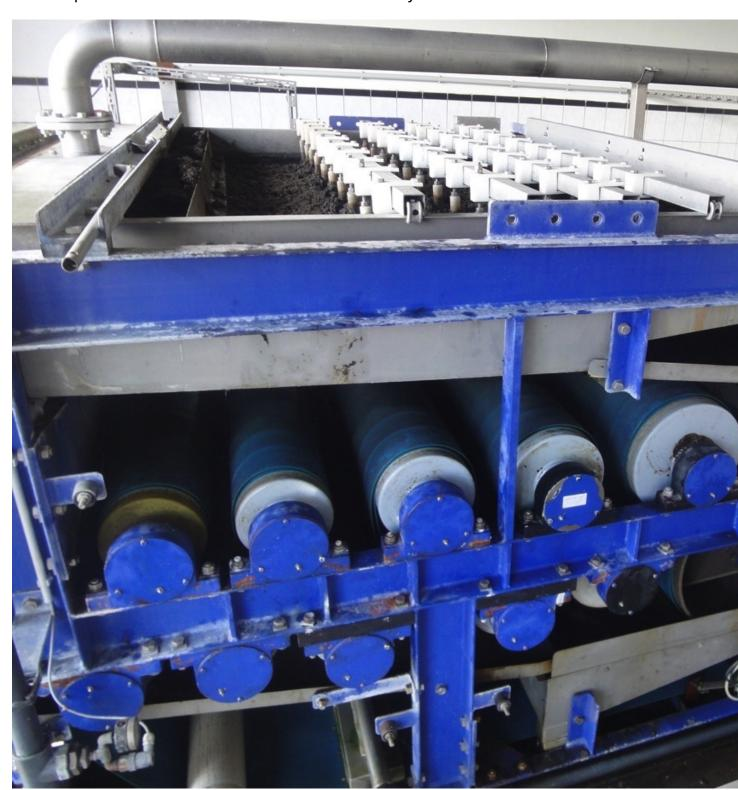
The belt press is fed directly from the thickener, so around 160 cubic meters of sludge is dewatered per day.
