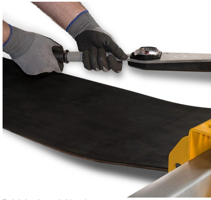
The belt clamp is securely tightened using a torque wrench. (Photo: Flexco Europe GmbH)
