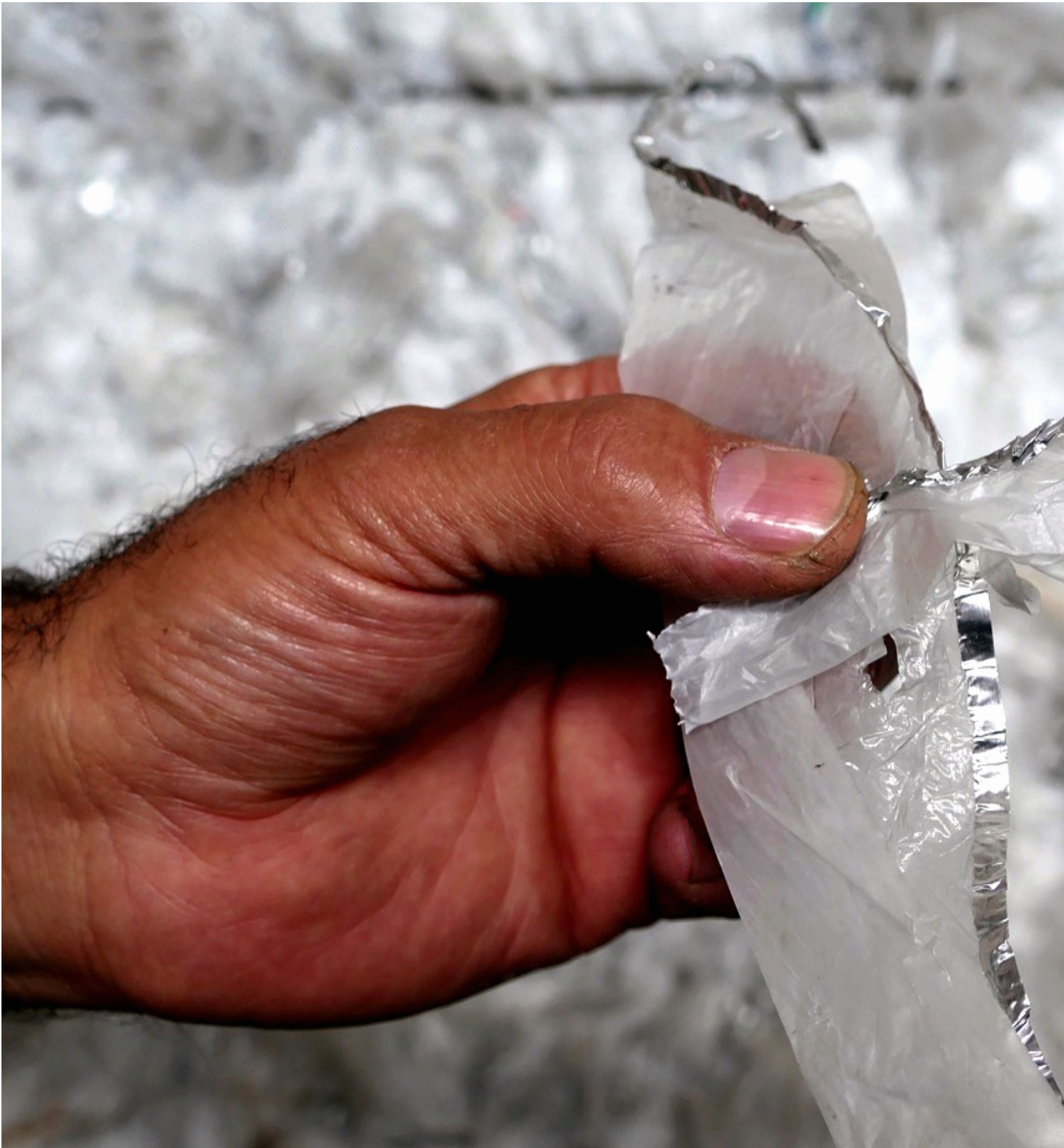
A lucrative material: edge trim with an aluminum fraction. The film scrap which typically occurs when beverage packaging is manufactured from laminated carton is shown here. (Picture: ETTLINGER)
