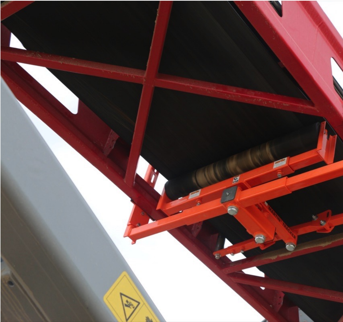
The Roller Tracker centers the cargo, reduces spillage and increases safety.
