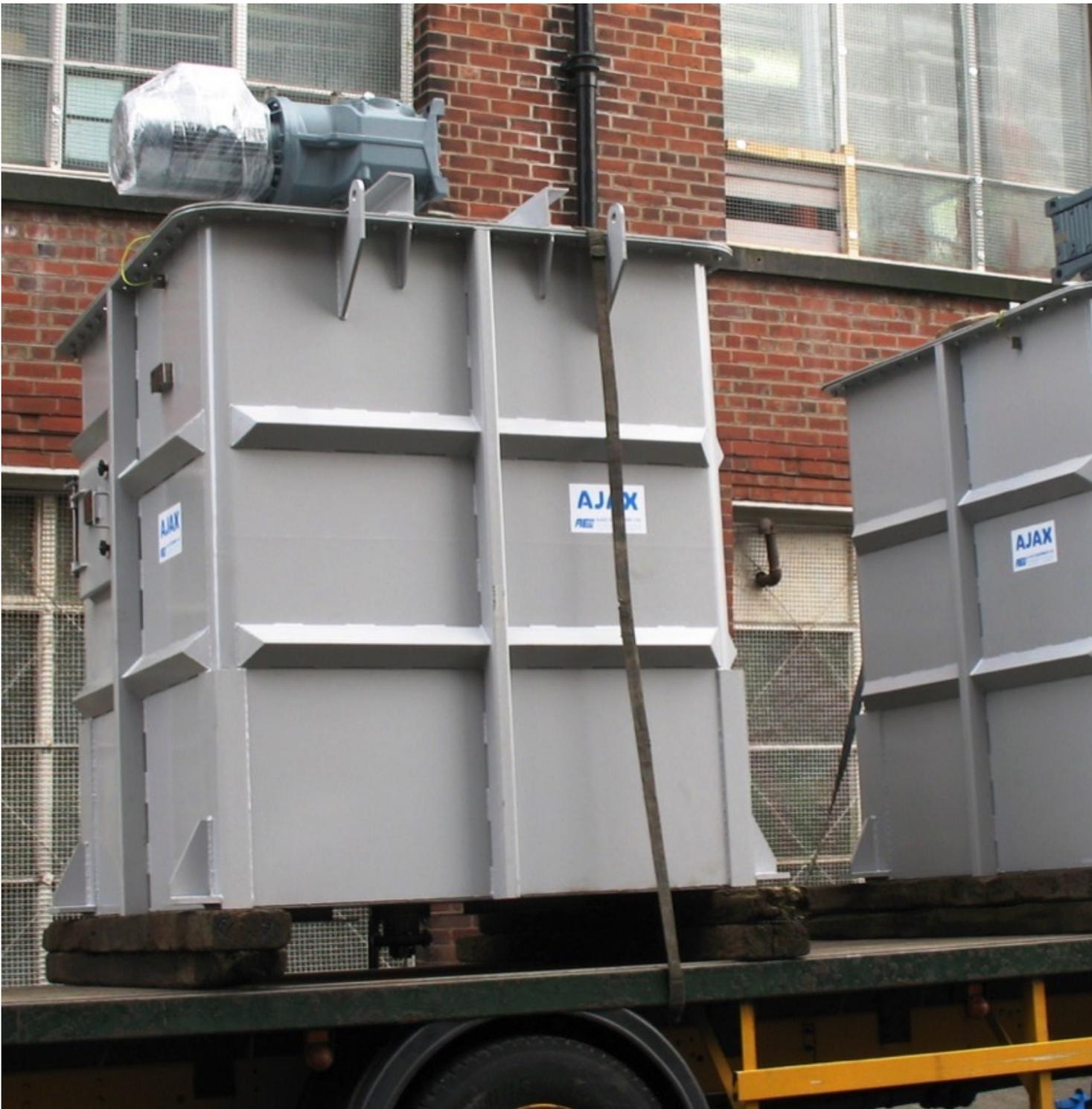
Two Ajax Cascade Mixers, 5.5 metre cube capacity site rated Atex zone 21, internal Zone 22.
