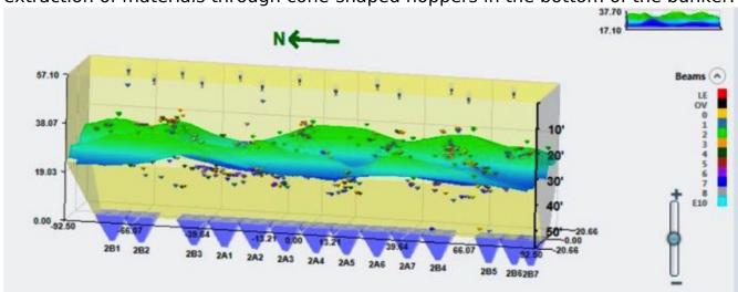
In proven installations, up to 20 3DLevelScanners have been mounted in the upper structure of the bunker roof. The bunker is virtually divided into sections as small as 1.5 by 1.5 meters with the 3D sensors continuously measuring changes across the surface and providing unique visual and data reporting of inventory in
