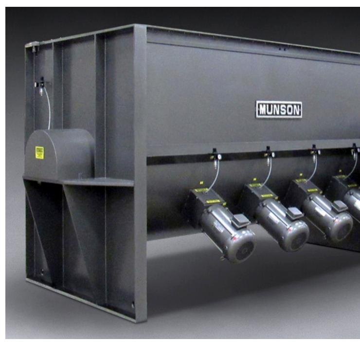
Munson Model HD-510-MS Paddle Blender is equipped with four highspeed choppers.
