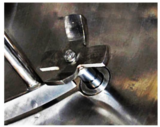
The paddle agitator forces material into the path of the tulip-style, high speed choppers, breaking down agglomerates and lumps for dispersion into the batch.
