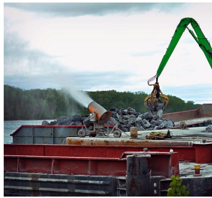
The mist can be seen stretching across the deck to deliver efficient dust suppression.
