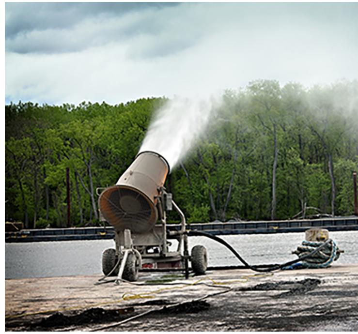
The unit features a 200-foot reach, 359° oscillation and 50° vertical adjustment angle.
