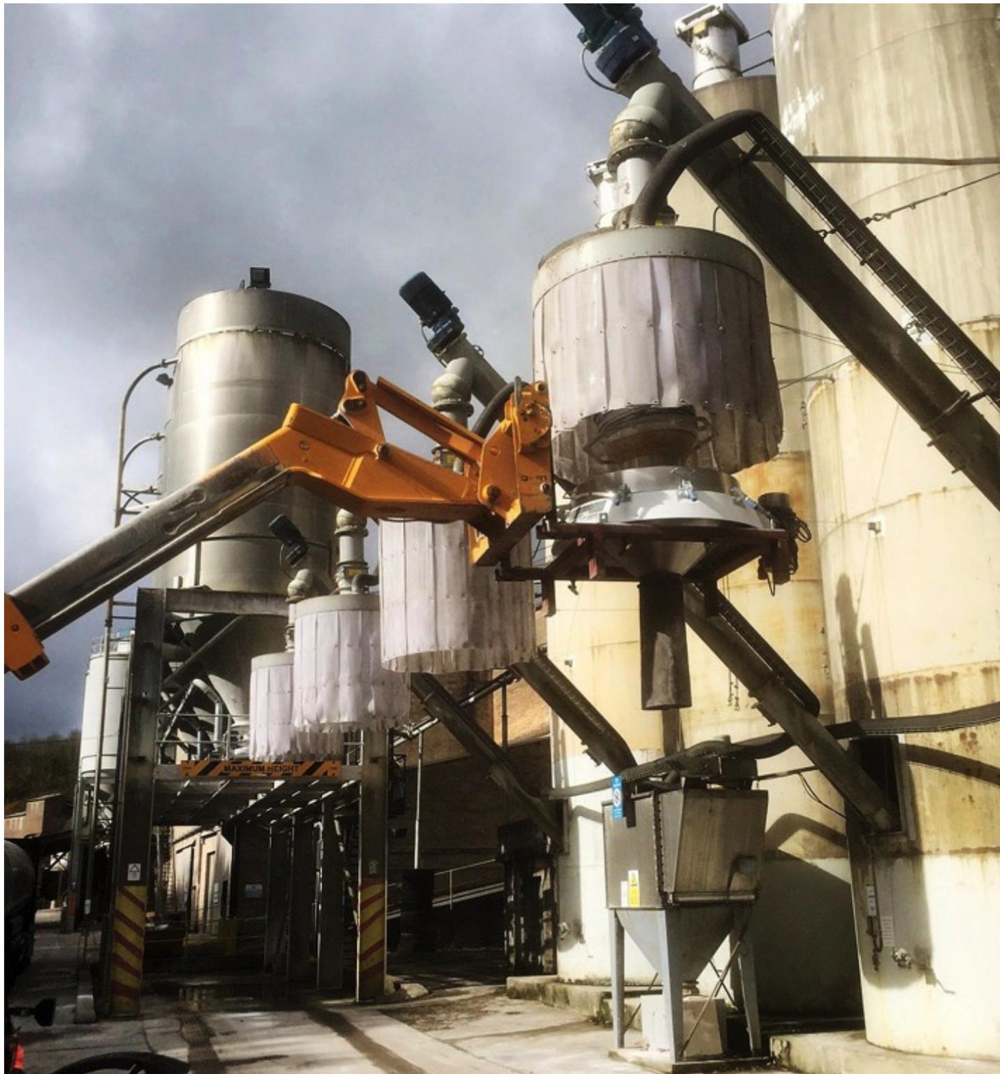
The sieve unit is transported and elevated into position above the tanker using a telescopic handler.
