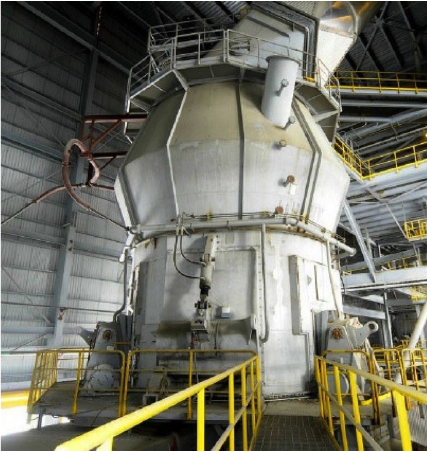
Example of a LOESCHE mill type LM 53.3+3 CS.
