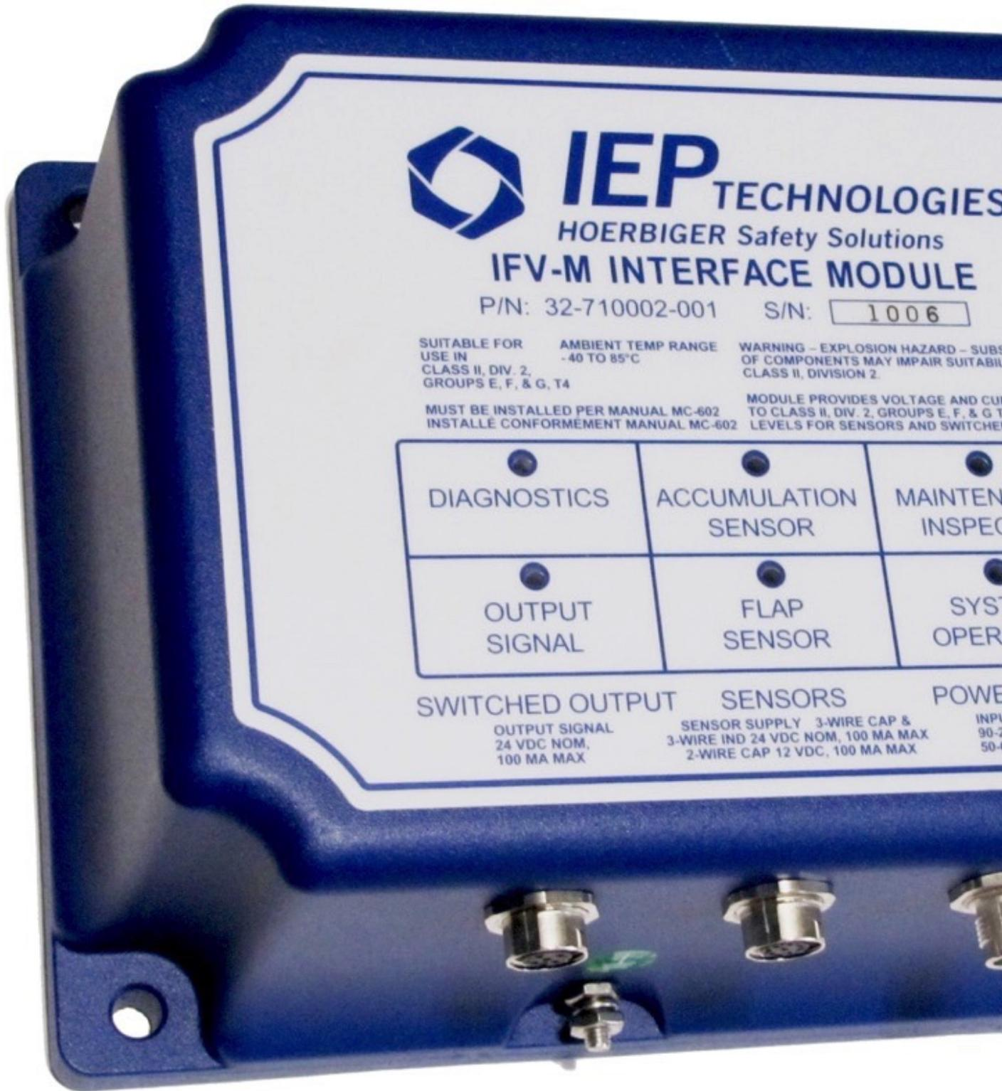
The IFV-M interface module can provide notification and process interlock if the isolation flap valve is closed due to an explosion or material build-up. (Picture: HOERBIGER)
