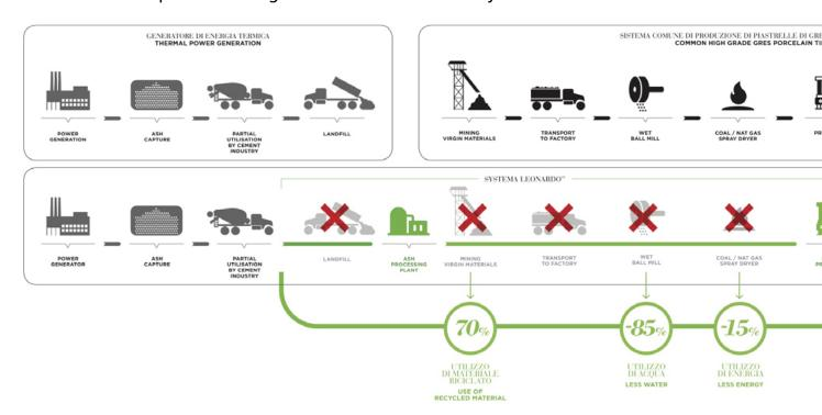
Vecor's Systema Leonardo facilitates the cleaning up of waste left by power stations and the conversion into high value products.
