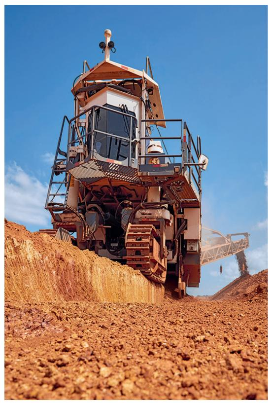
During the mining process, Wirtgen machines produce level surfaces that serve as stable roadways, facilitating rapid transportation of the mined material. During this process, the LEVEL PRO leveling system collects and transmits data on the leveling process
