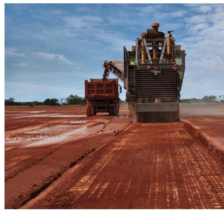
Wirtgen surface miners can do much more than just extract pay minerals. In Guinea, they are also used to open routes and develop the infrastructure around the mines.
