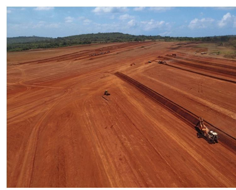
Wirtgen's 2500 SM sidecasts the mined material, producing high windrows. The leveled sidecast material is clean, stable and ready to be transferred onto trucks with wheel loaders or excavators.
