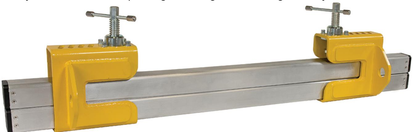
The 6-ton clamps are available for belts up to 72" (1800 mm) wide and up to 2" (50 mm) thick, while the 8-ton clamps are available for belts up to 96" (2400 mm) wide and up to 2 1/4" (55 mm) thick. TUG HD Belt Clamps are also versatile, portable, and easy to use. A single pair of the easy-to-carry heat-treated
