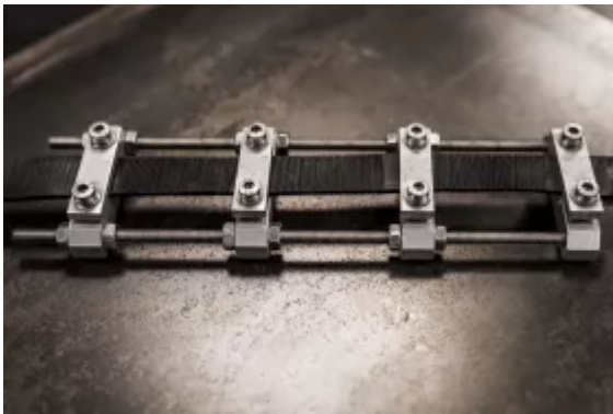
ISO 1431. Lateral cracking. The effects of ozone on rubber.
