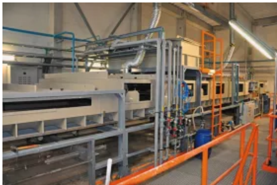
Fig. 1: A BHS belt filter system in the Holcim factory located in Rohoznik, Slovakia.
