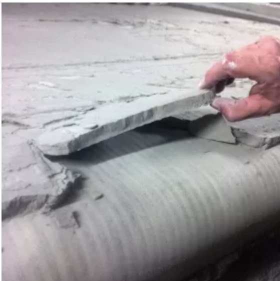
wp_2428.jpg Fig. 5: The pre-dried filter cake is crumbly and can be transported away on a conveyor belt.
