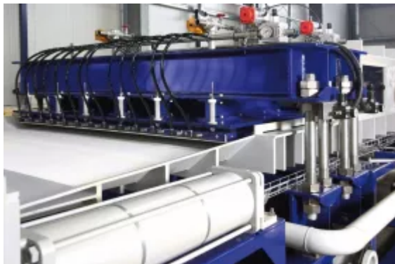
Fig. 4: Various dewatering systems can be used to dry the filter cake. Mechanical compression is possible with the optional pressing device, together with a blow-out, if applicable.
