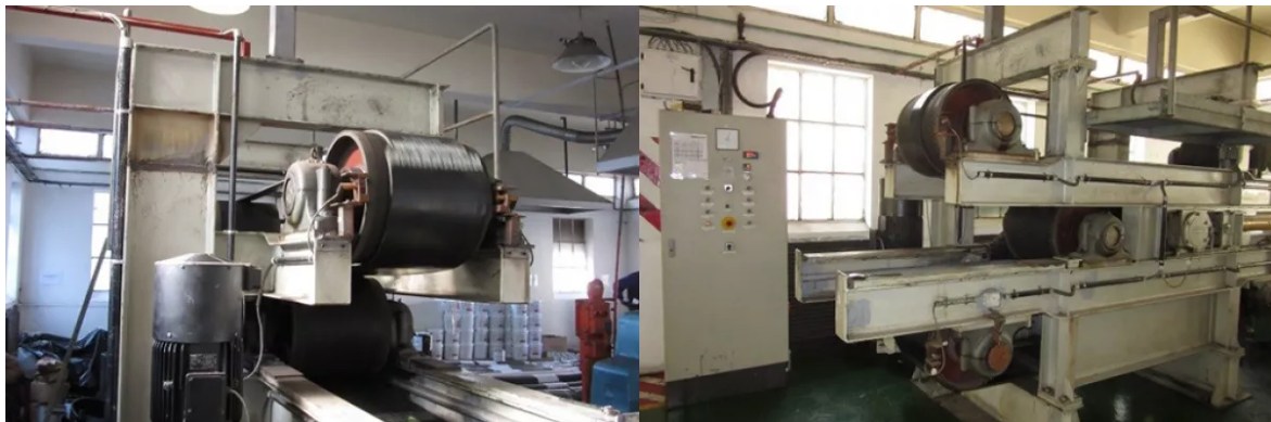
Fig. 6: DIN dynamic splice testing equipment
