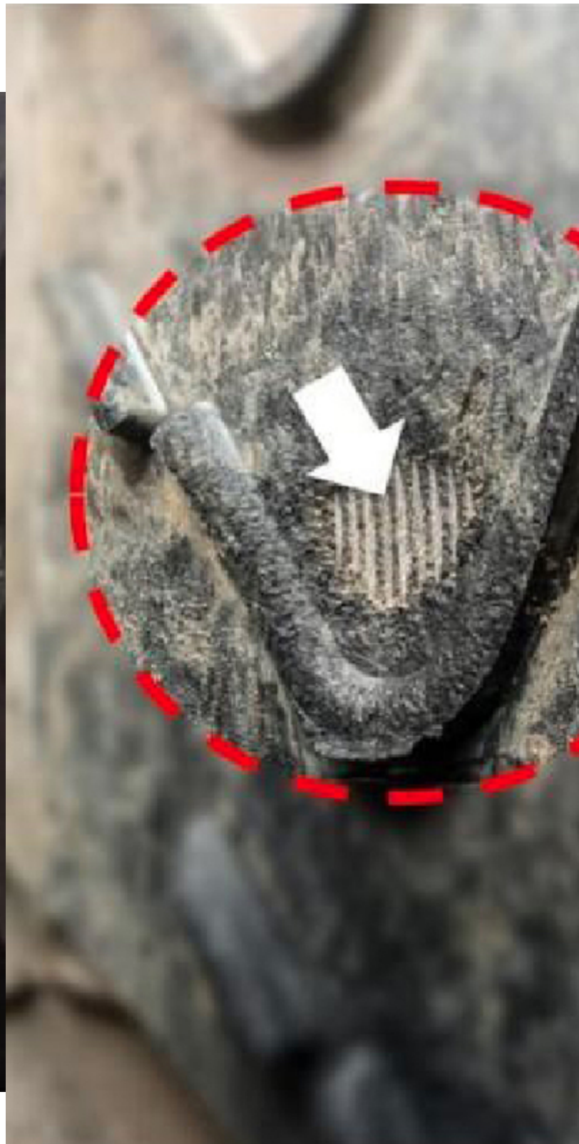
Fig. 8b: Experimental investigations of the impact-strength, bond-strength and wear-resistance of the new chevron cleat ribs in a belt system transfer station in the Oetelshofen limestone opencast mine.
