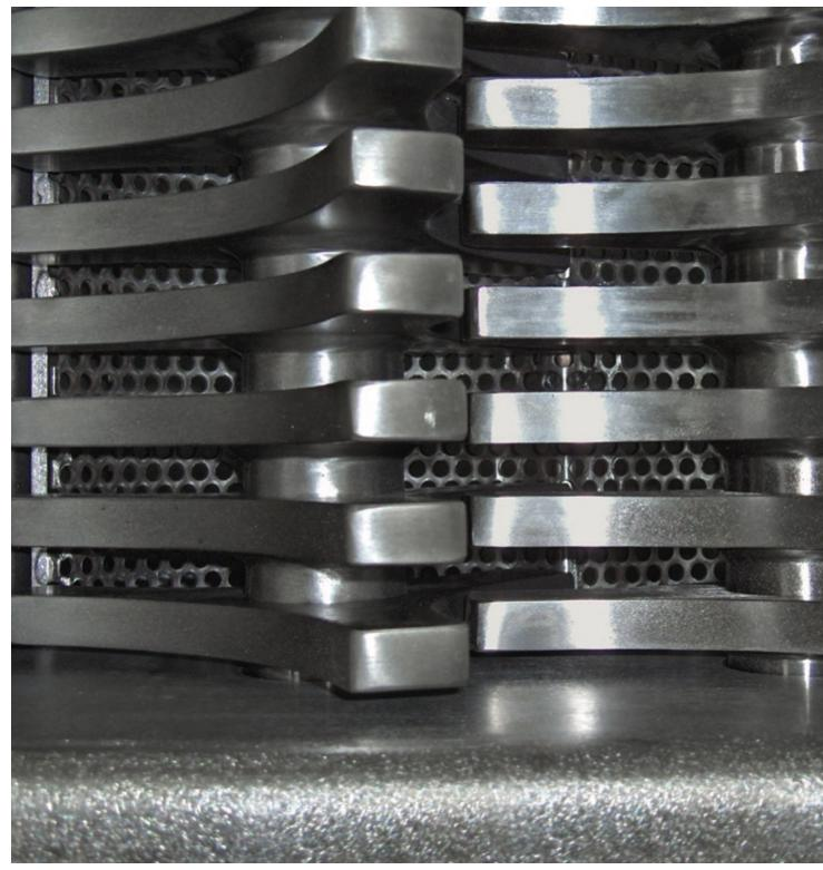
Dual rotors with three-point, singlepiece, abrasion-resistant breaking heads rotate with minimum clearance inside a curved, perforated bedscreen with apertures from 25 to 64 mm in diameter.
