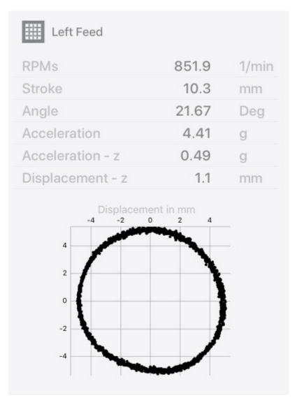
The app-controlled vibration analysis sensor enables readings of screen box vibrations within seconds and generates a report that can be sent or reviewed.
