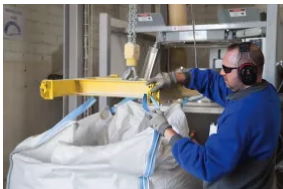
Operator delivers bulk bag, and attaches bag loop straps to the lifting frame. (Pictures: © Flexicon Corporation)
