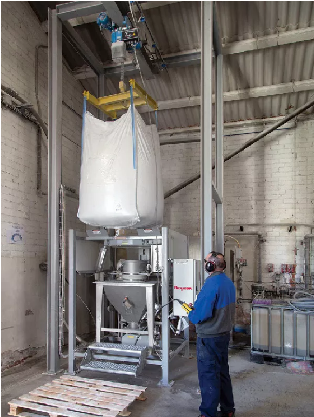
The cantilevered hoist and trolley position the bag for discharge into the 226 l hopper and through a rotary valve into the pneumatic line.
