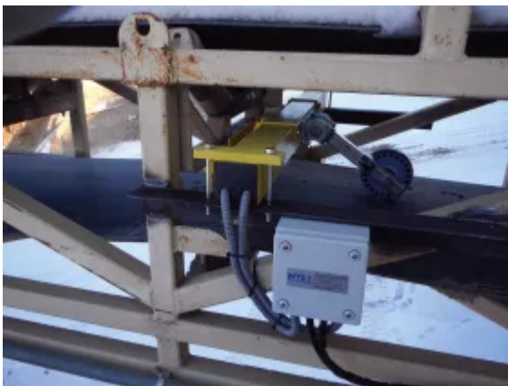
Fig. 2: ESW 2.2 belt scale installed in a conveyor for measuring the transported dolomit bricks.
