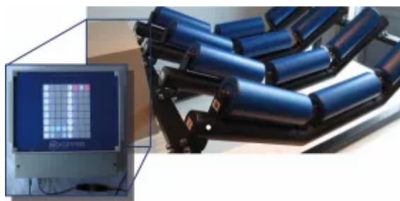
Fig. 1: Demonstration model of sensing idlers with AKT monitoring system. (Pictures: © Artur Küpper GmbH & Co. KG)
