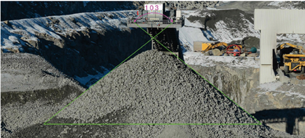
Fig. 10: Angle of surcharge of a copper ore heap in reality (l.) and in the DEM model (r.). (Picture: © Contitech AG CBG)
