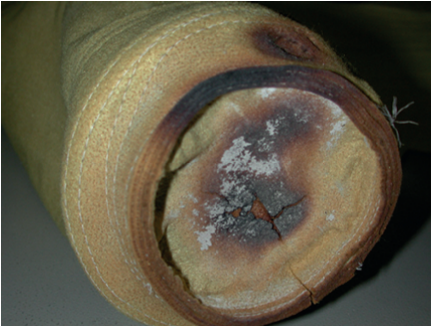
Fig. 5: Shrunk bag bottom as a result of high hopper dust levels.
