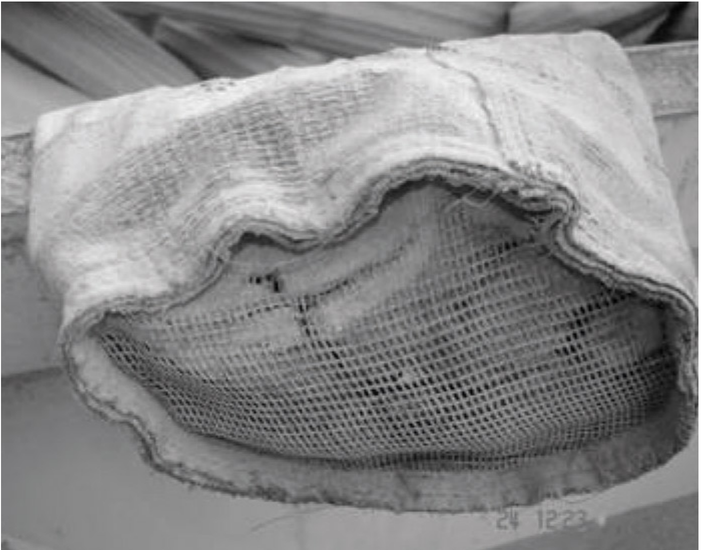
Fig. 6: Abrasion of the entire felt from the supporting scrim due to high local gas velocity.
