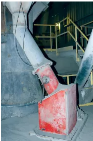
Fig. 4: St. Marys Cement in Canada has been using the Siemens E-300 solids flowmeter for over two decades.
