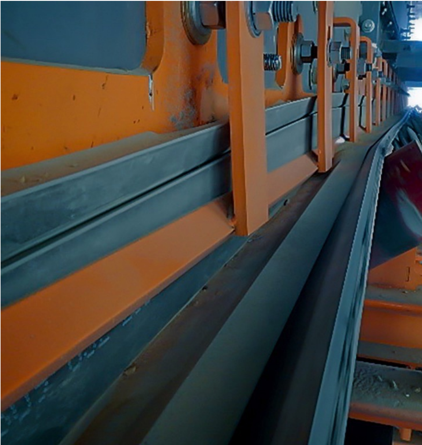
Fig. 3: Impact cradles absorb the force of the falling load, yet slide in and out for easy service. (Picture: © Martin Engineering)
