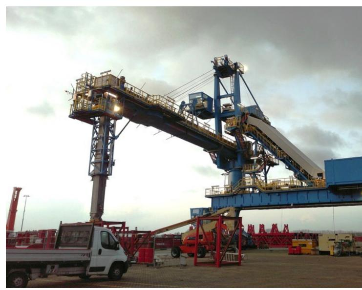
The DSI Sandwich high angle conveyor will transfer urea and amidas prills at a rate of 600 t/h at a 45° angle.
