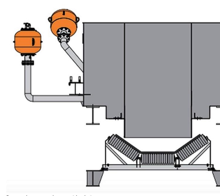
Proper air cannon placement in chutes and silos can reduce ongoing buildup. (© Martin 2020)
