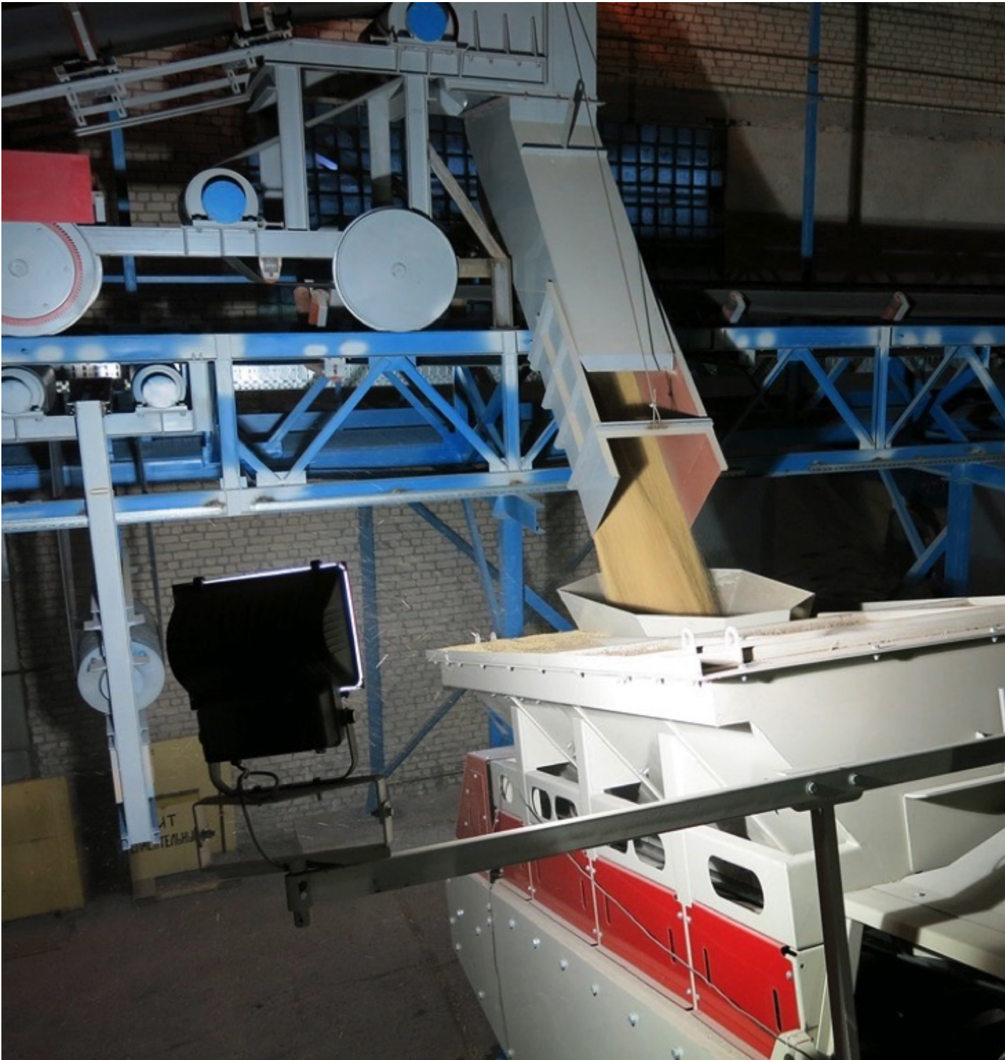
Grain being fed to the custom designed TS 550 shiploader. (Pictures: ©Telestack Ltd.)
