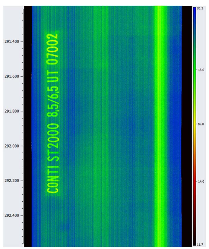
On the basis of the data recorded, Conti SurfaceInspect creates a digital map on which all cover plate damage is visible.
